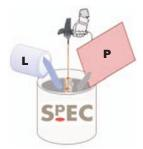
Add approximately 50% of the liquid component to a clean 25 litre steel drum and gradually add the powder whilst mixing using a slow speed heavy duty drill fitted with a suitable
